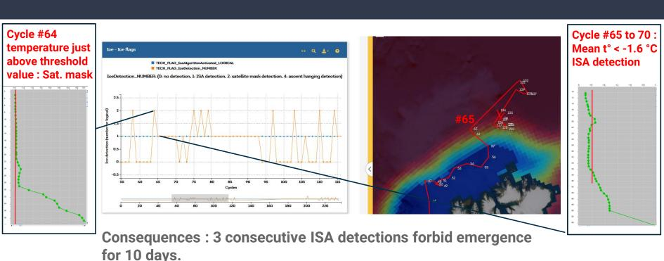
Then No ISA detection an no Sat. Mask for 10 consecutive days allow float to surface @ cycle # 101.
