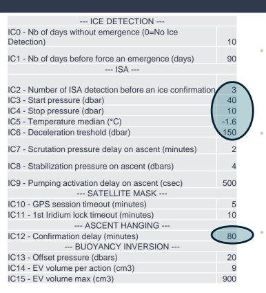
Adjustment of the temperature threshold to -1.6°C (Default= -1.78°C, Baffin bay = -1.3°C)
