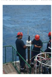
CHECK LIST 1: Get the float out of the box and put it safely in vertical position on an outside open deck (necessity for the float to perform a GPS / Iridium satellite fix when activated)
