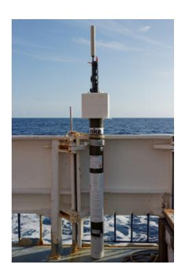
CHECK LIST 2: Remove the 3 red protective plugs from the float's CTD head (otherwise float won't work as these are the water intakes for temperature and salinity measurements). For float with optodes, remove black optodes's cap.
