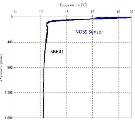
Temperature time series have similar shapes for both NOSS and CTD sensors from 0 to 2000 dbar  $\delta T$ <0.01°C
