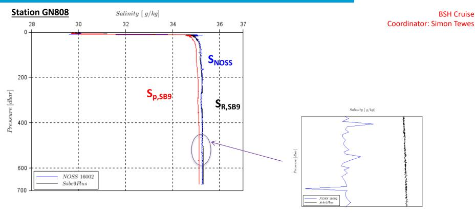
δS ≤ 0.03 g/kg due to disalignement in Temperature (to be corrected)
